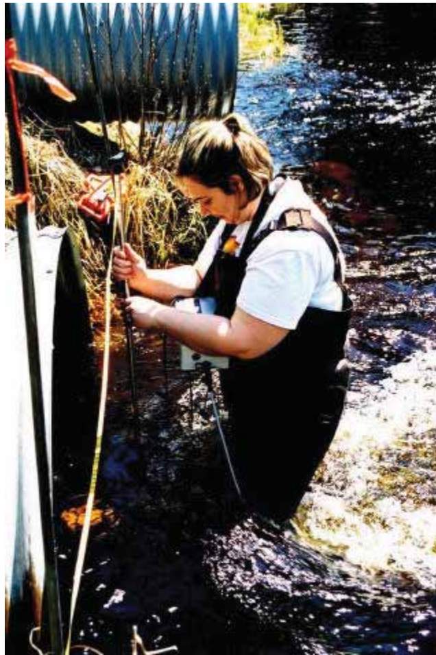
Figure 2. Allison Selinger measuring water velocity in the Black River at Hwy 314 in Nopiming Provincial Park.
