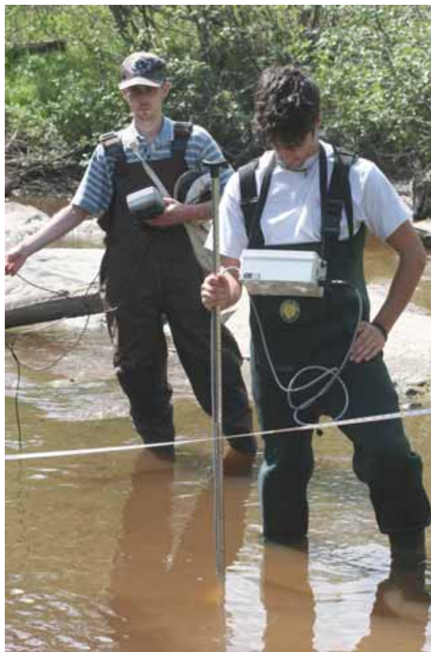
Figure 3. Summer student Daniel Dupont measuring water velocity (in foreground) and Matthew Doering measuring water temperature and dissolved oxygen.
